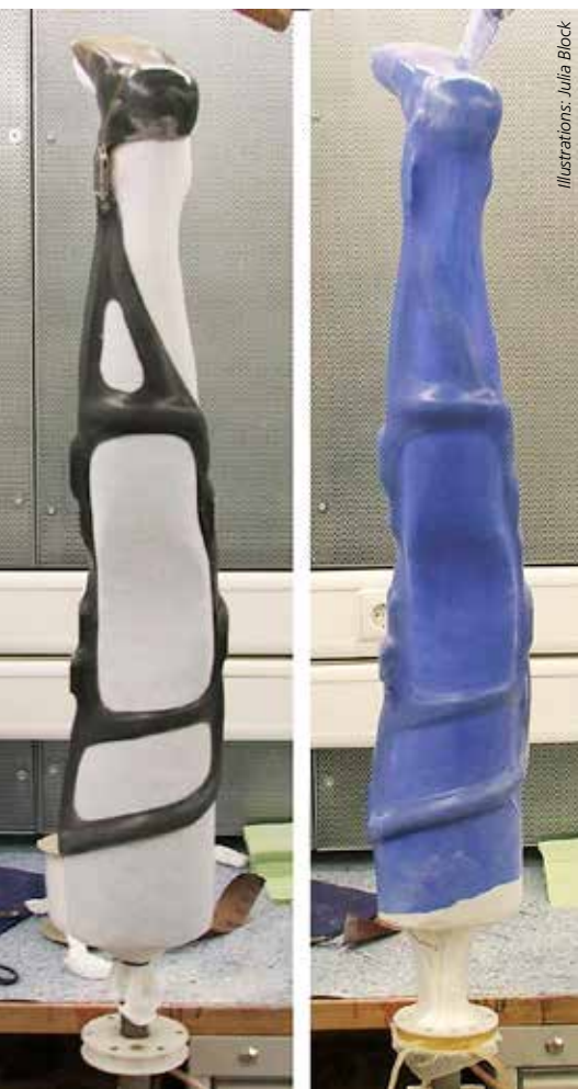
Building the orthosis with the help of fibre composite technology: a profiled carbon fibre framework is shaped around a plaster model of a volunteer's leg and resin soaks the fibre mesh, forming the braces.
