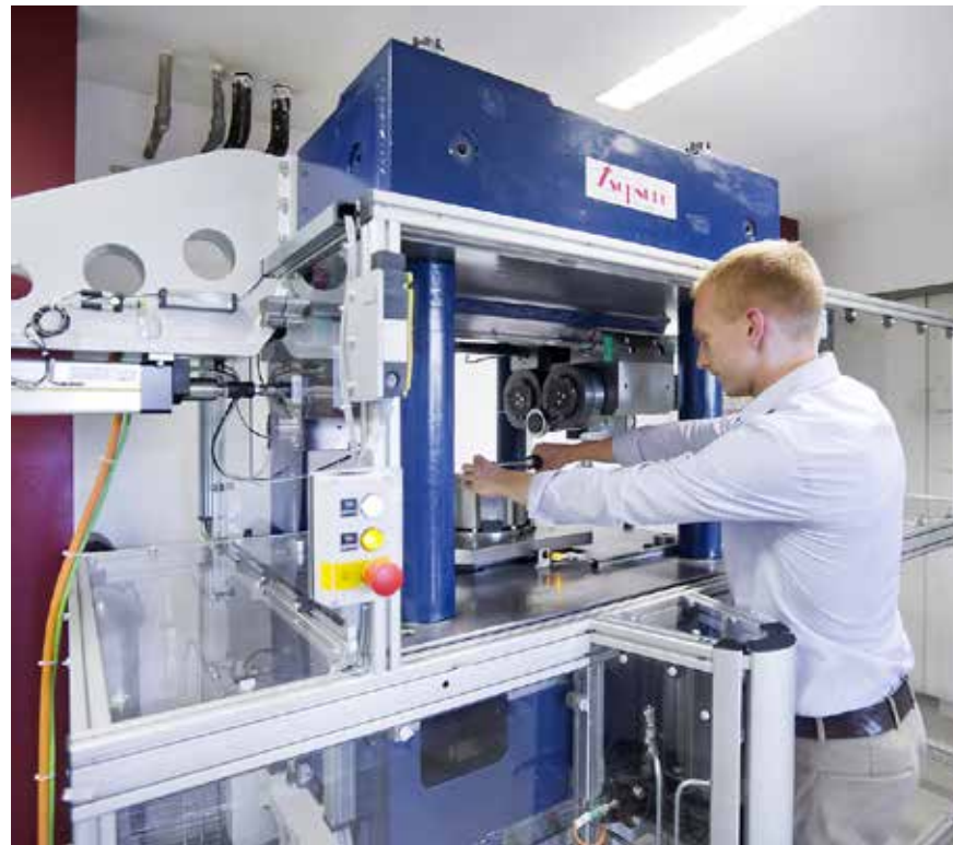
Above: Concentrated work on a flexible rolling system. Below: During rolling, the rotating workpiece is machined such that the material undergoes “process-adapted distribution”. Tool inserts allow a wide range of geometries to be created.
