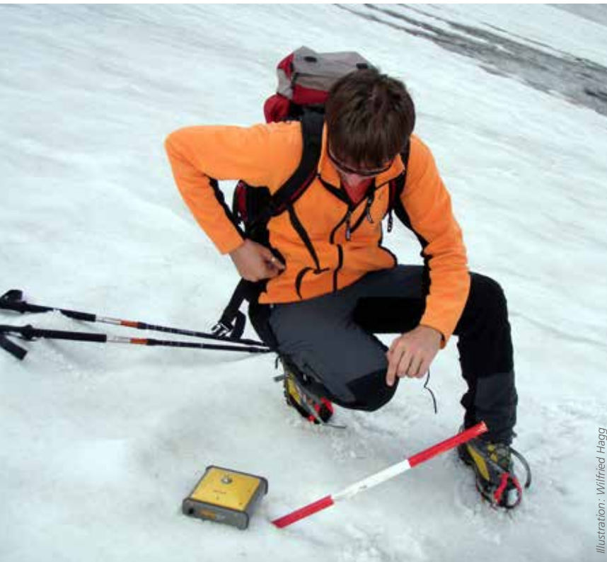
Above left: Taking measurements on the Blaueis, the northernmost glacier in the Alps, with a laser tachymeter. Above right: GPS surveying of a melt stake and (below) performing a radar survey of the Lupo Glacier.
