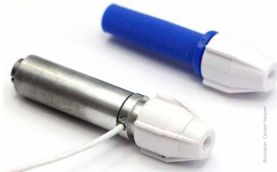
Top: Force sensor for the guide wire tip, shown here on a test board. Right: The handheld tool, known as a torquer, with integrated force sensor, shown with a conventional model for comparison.
